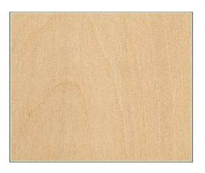
**GRADE BB** - One side is generally light and uniform in colour. Pin knots and small sound tight knots are allowed. Occasional football patches are colour matched to the veneer. Sanding is smooth, 100 - 120 grit.
