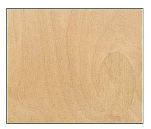
**GRADE CP -** One side is similar to grade BB in quality. Sound knots and patches may be more common that BB grade. Small open splits, knot holes and double patches are allowed. It may have some streaks and discolorations. Sanding is smooth.
